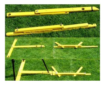
The tactile sighting aid comprises two parts, a stand and the tactile device itself. Stands are typically adapted from photographic tripods, music tripods, or similar. The purpose of the stand is to enable the tactile device to be moved up and down so that adjustments in elevation of the bow can be achieved.
